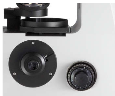
Camera connection and coaxial coarse and fine focusing knob
